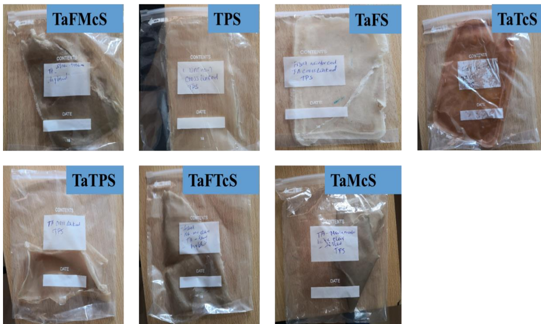
Figure A 6 samples prepared from tartaric acid modified, cellulosic fiber and clay reinforced
